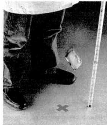
DROP TEST After a 5-foot fall onto concrete, the Tough-6000 was unscathed.
